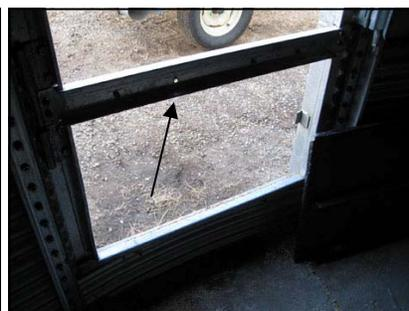
Open bolt hole in center bar
