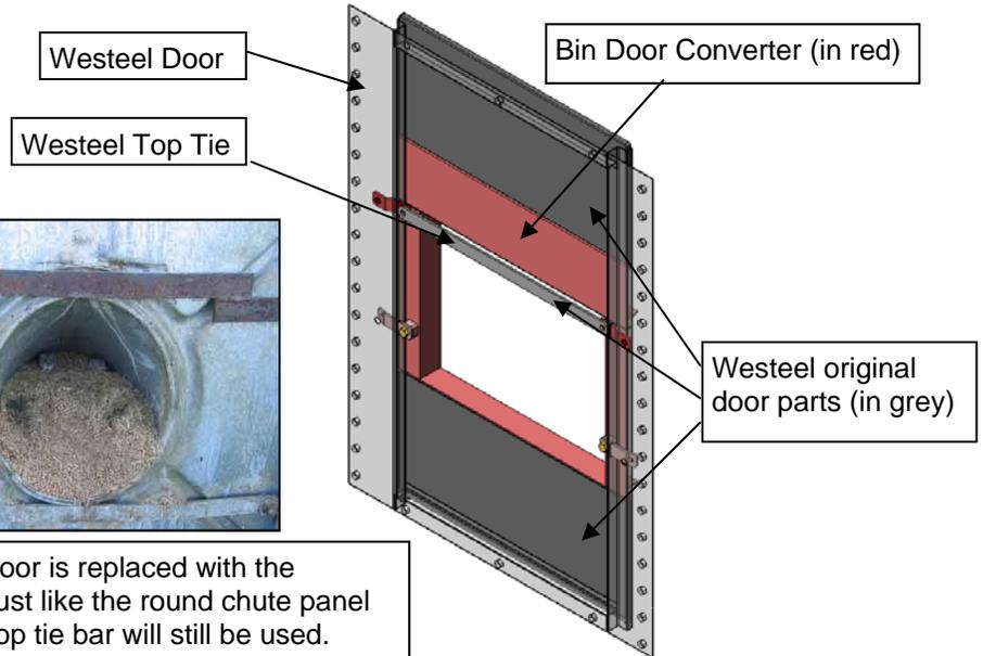
The round chute panel that came with the door is replaced with the converter. The converter slides into place just like the round chute panel did and the BDI fits to the converter. The top tie bar will still be used.
