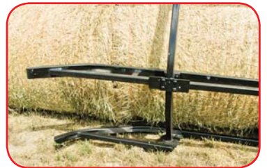
As the bale ends touch, completely lower the chambers and back out.
