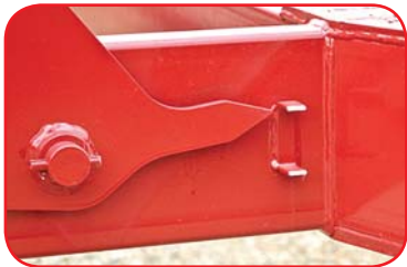
Pointer helps you know when chamber is in loading/unloading position.
