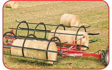
When bale(s) are in position, partially raise the chamber.
