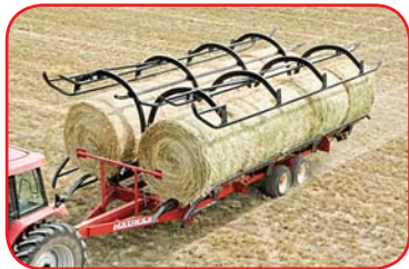
Raised chambers, with front and rear bale stops, help contain load.
