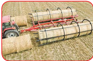
Start lowering the chambers as you drive into your unloading area.
