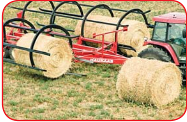
With the chamber still slightly raised, line up the next bale.
