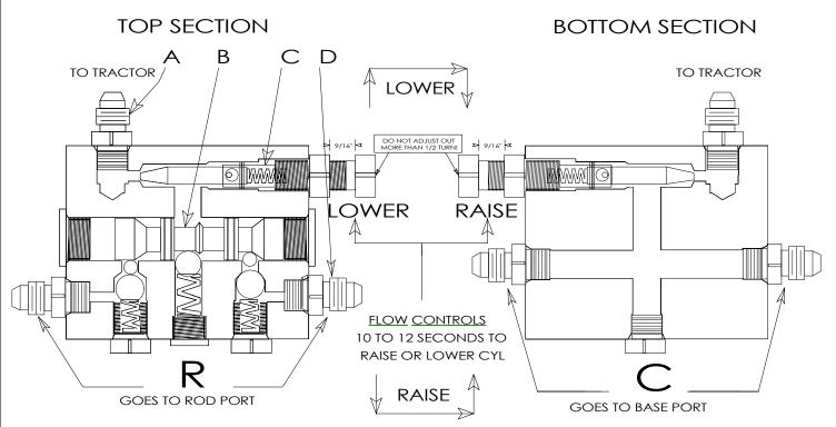
The following are the instructions for plumbing a SHOEMAKER Sequencing Valve with the SIDE ARM Field Markers.
