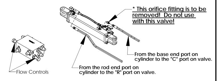
\* - The orfice may reduce the oil flow to much and may not allow the valve to cycle as it should. Remove the orfice and control the folding speed with the flow controls on valve.
